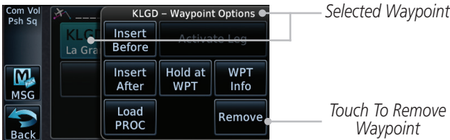
Figure 4-4 Remove Single Existing Waypoint
