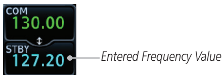
Figure 3-18 Completed Frequency Entry
