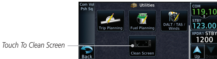
Figure 14-47 Utilities Home Page
