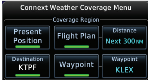
Figure 11-58 Connex Weather Coverage Region Menu
